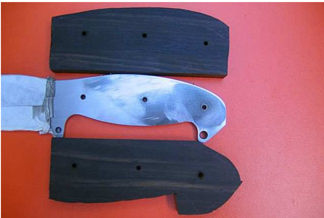
Ecco le guancette forate. Here the drilled slabs
